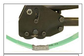
Your final seal should be flat and completely sealed as the image above shows!
