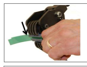
Make sure that small overhanging side of the seal should match up with the smaller (upper) side of the sealer.
