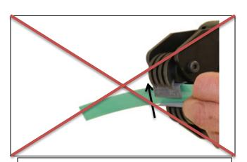
Your seal should not look like the above image where the large overhanging side of the seal is matched up to the smaller (upper) side of the sealer!
